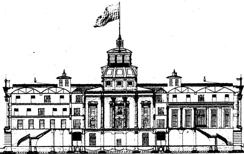
NEW CUSTOM HOUSE at NEW ORLEANS, LA SECTION FROM CANAL STREET to CUSTOM HOUSE STREET.
