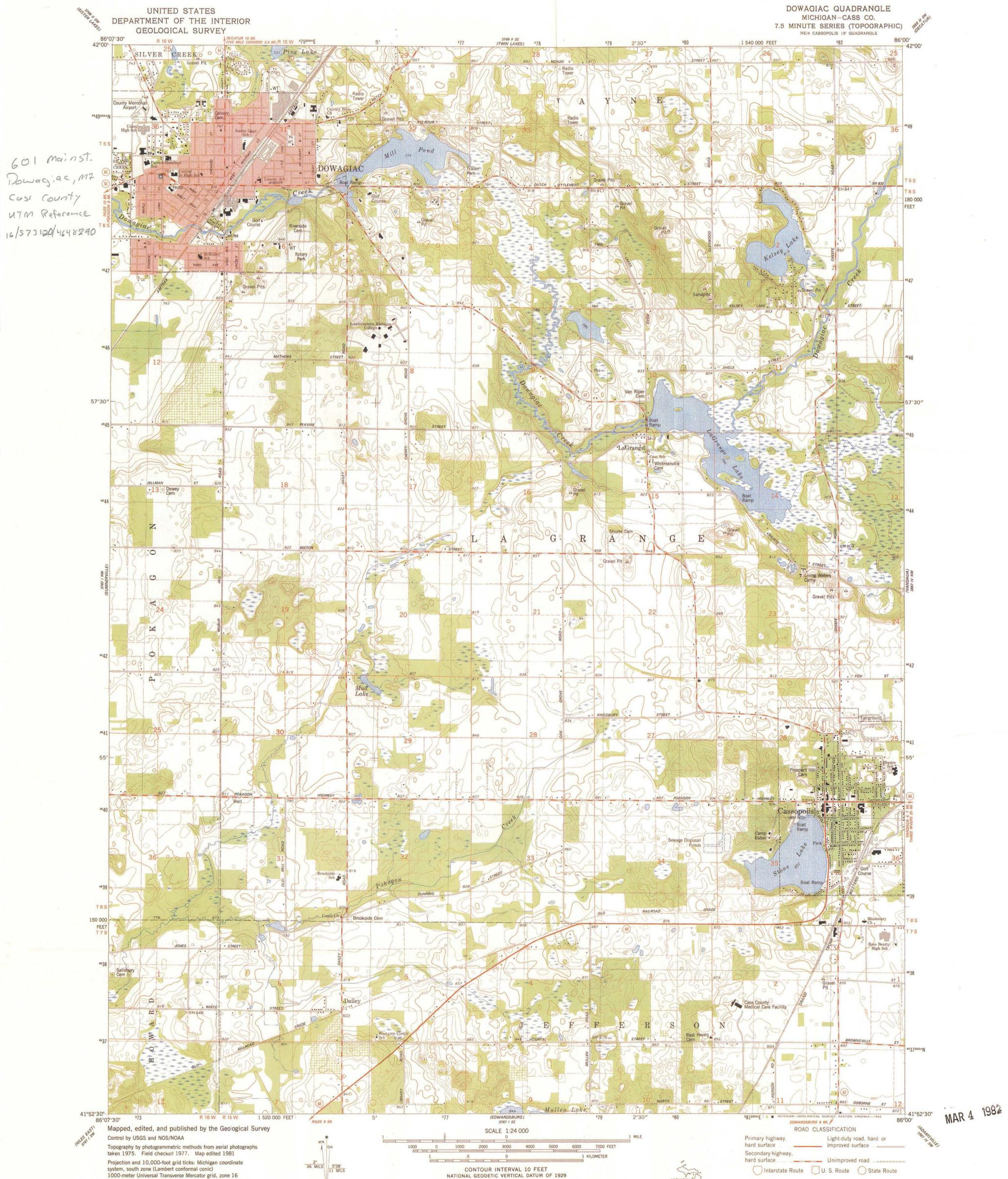
1000-meter Universal Transverse Mercator grid, zone 16 1927 North American Datum To place on the predicted North American Datum 1983 move the projection lines 1 meter north and 2 meters east as shown by dashed corner ticks Red tint indicates areas in which only landmark buildings are shown Fine red dashed lines indicate selected fence and field lines where generally visible on aerial photographs. This information is unchecked
