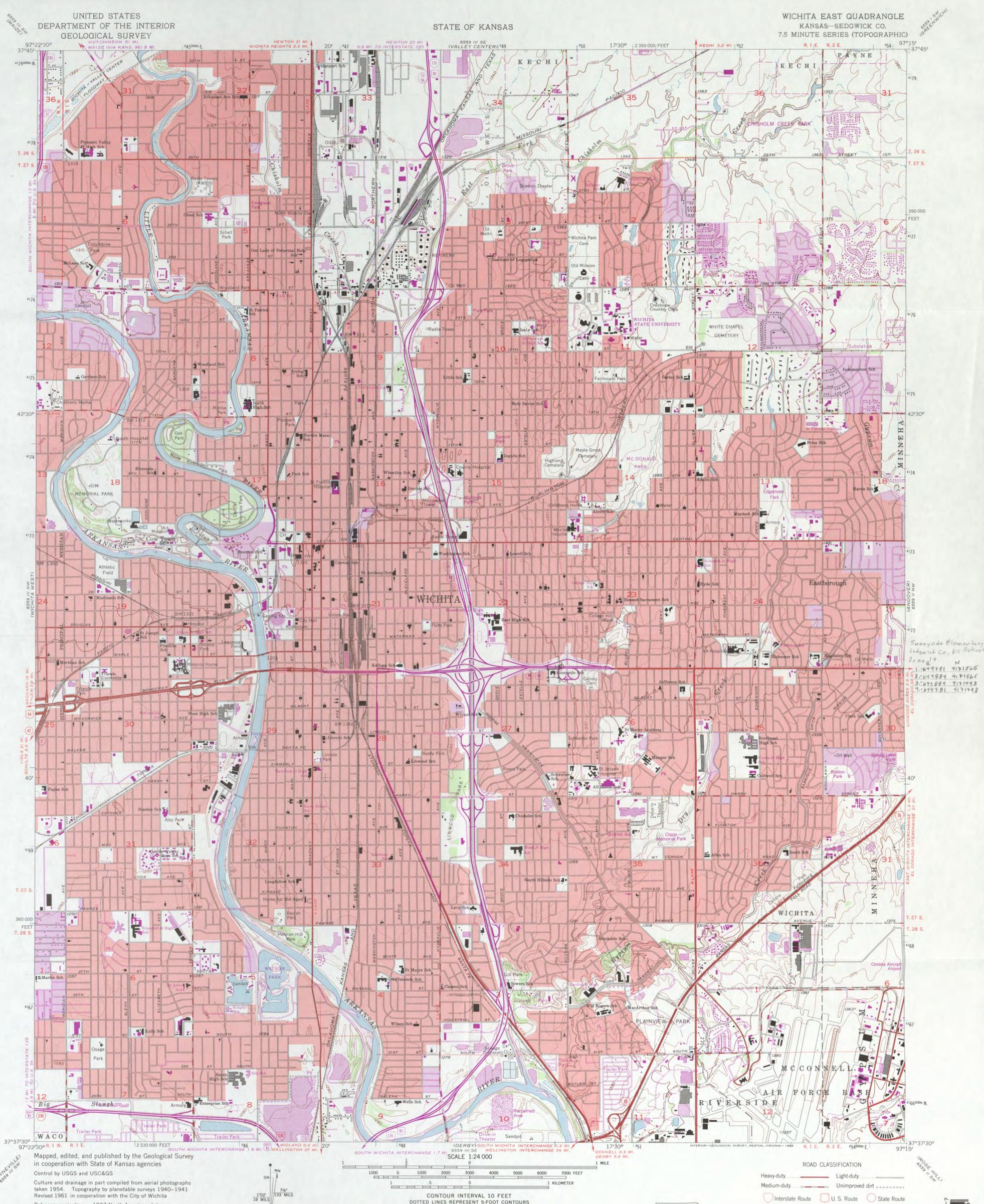
taken 1954. Topography by planetable surveys 1940–1941 Revised 1961 in cooperation with the City of Wichita Polyconic projection. 1927 North American datum 10,000-foot grid based on Kansas coordinate system, south zone 1000-meter Universal Transverse Mercator grid ticks, zone 14, snown in blue
