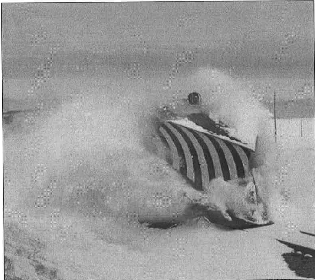
Figure 2. The cover of the Streamliner pictured UP wedge plow number 900015 in action clearing track near Strasburg, Colorado, in 1982. SOURCE: Streamliner 6(1992).
