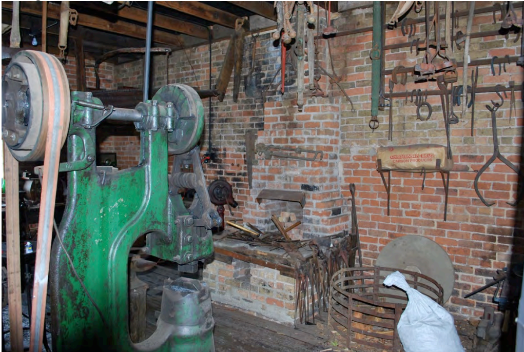
14 of 17: Interior view of western-most forge with power hammer in foreground. Camera facing northwest.
