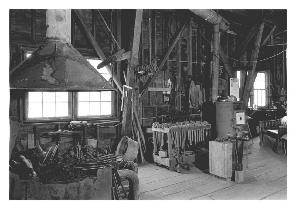
9 of 13 Interior view: looking SE from east side of lower story Note forge in foreground; timber bracing for reinforced floor above
