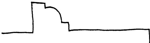
door trim, second floor, room side, hall door
