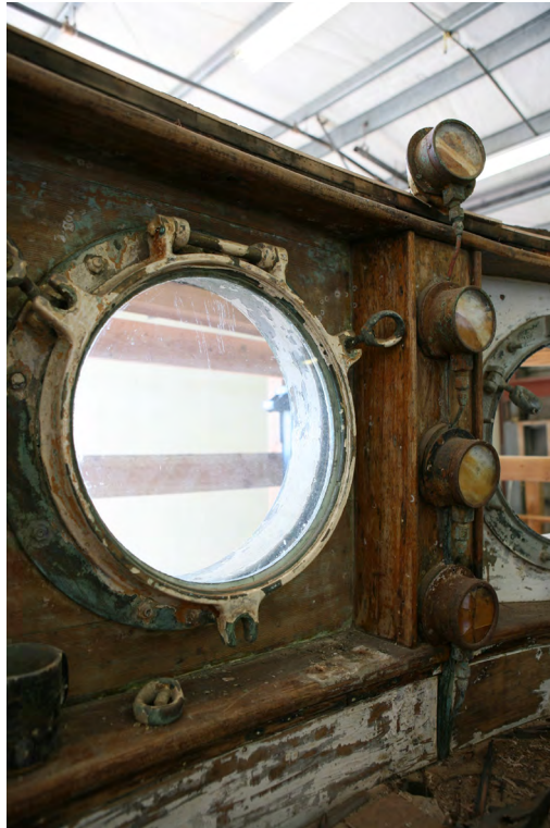
15 of 20. Western Flyer. Wheelhouse, detail view of port lights and former gauges.
