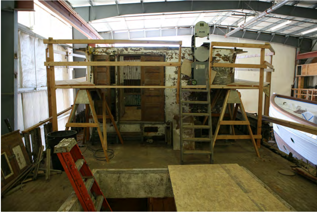
5 of 20. Western Flyer, at the Port Townsend Shipwright's Co-op, Port Townsend, WA. Looking forward, showing the rear of the deckhouse, from midship. Main hatch to fishhold in foreground. Note scaffolding and bracing, as part of restoration work ongoing in 2016.
