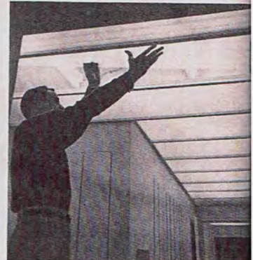
Ceiling-light strip starts here by the entrance, continues down hall to end bedroom (sketch low). Lightweight panels of white corrugated plastic are set in flush below fluorescent.
