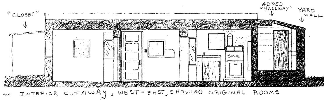
AA INTERIOR CUTAWAY, WEST-EAST, SHOWING ORIGINAL ROOMS
