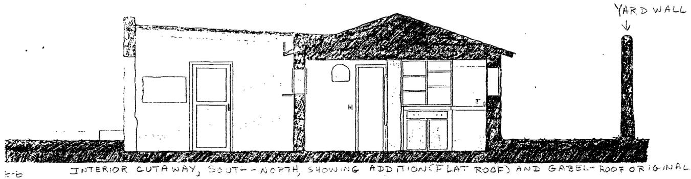
BB INTERIOR CUTAWAY, SOUTH-NORTH, SHOWING ADDITIONS (FLAT ROOF) AND GABLE-ROOF ORIGINAL
