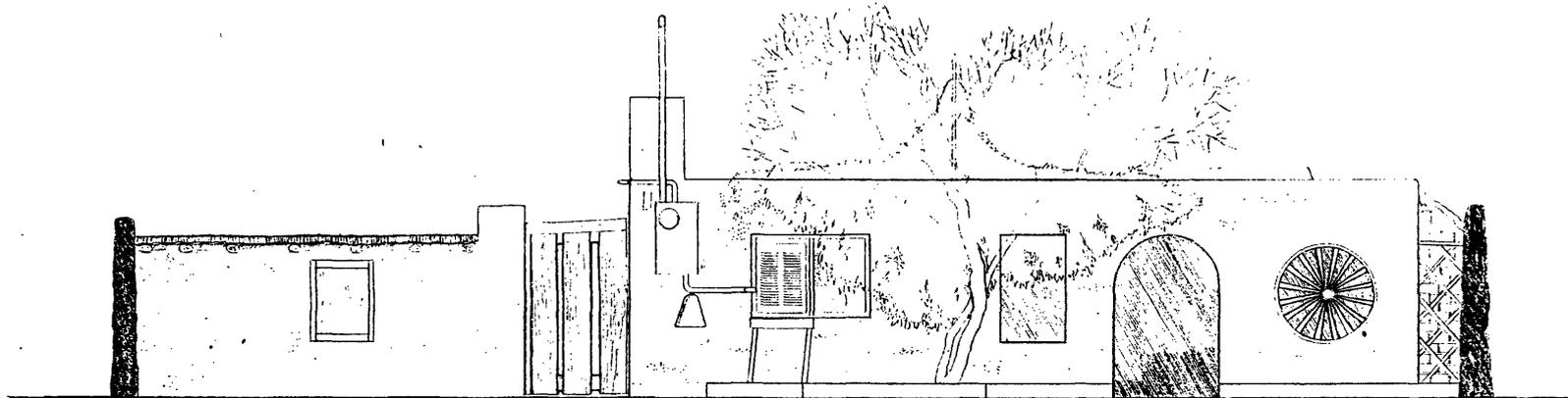
SOUTH FACADE, SHOWING PLASTERED MASONRY ADDITIONS
