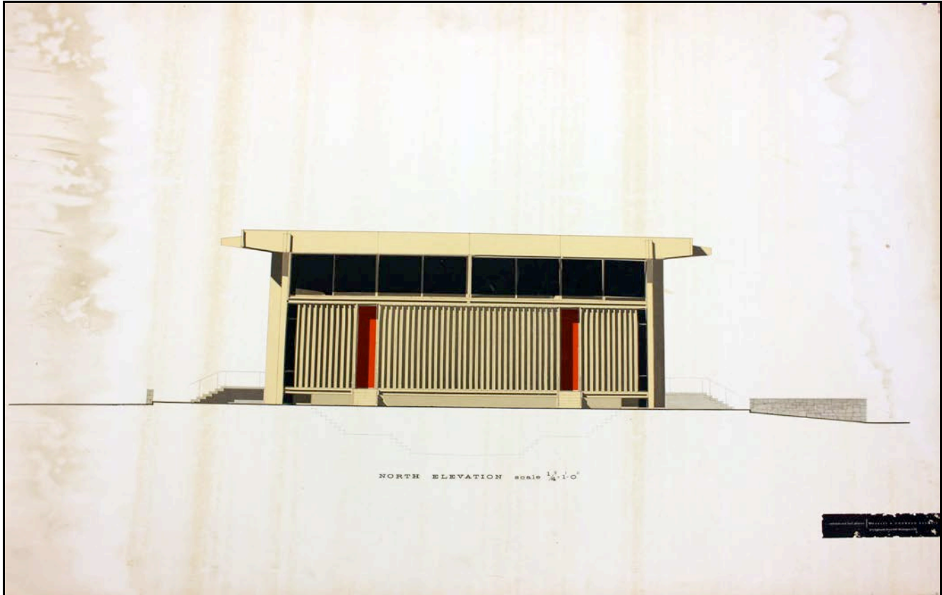
Image 10: North Elevation, Presentation Board, ca. May 1960, Charles M. Goodman Associates. This presentation board shows the north elevation of the Sanctuary, including each of the elements constructed and still intact today, such as the broadly overhanging roof, the clerestory windows, the corrugated wall panels highlighted by narrow fixed windows, and the two narrow, flush doors flanking the interior platform space. From the Archives of the Unitarian Universalist Church of Arlington.
