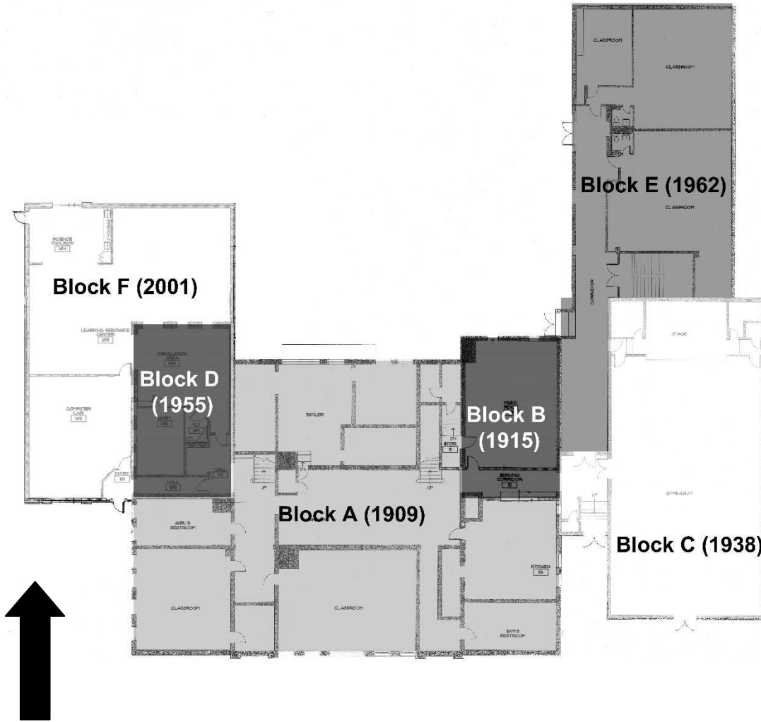
Figure 7. Hall School Blocks A-F (Basement Floor Plan).
