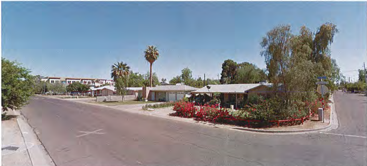
Figure 4. Houses within the Suburban Acres subdivision, view southeast from the intersection of 3 rd Ave. and Hazelwood Ave. This photo illustrates the change from pre-World War II era vertical curbing to rolled curbing typical of post-war development. Source: Google, 2016.
