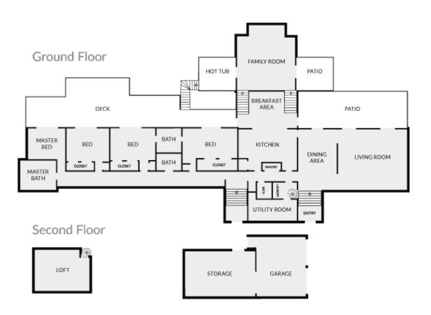
Floor plan of the Dr. James Patrick House. The shaded areas are parts of the house under roof. The second floor loft is located above the utility room.
