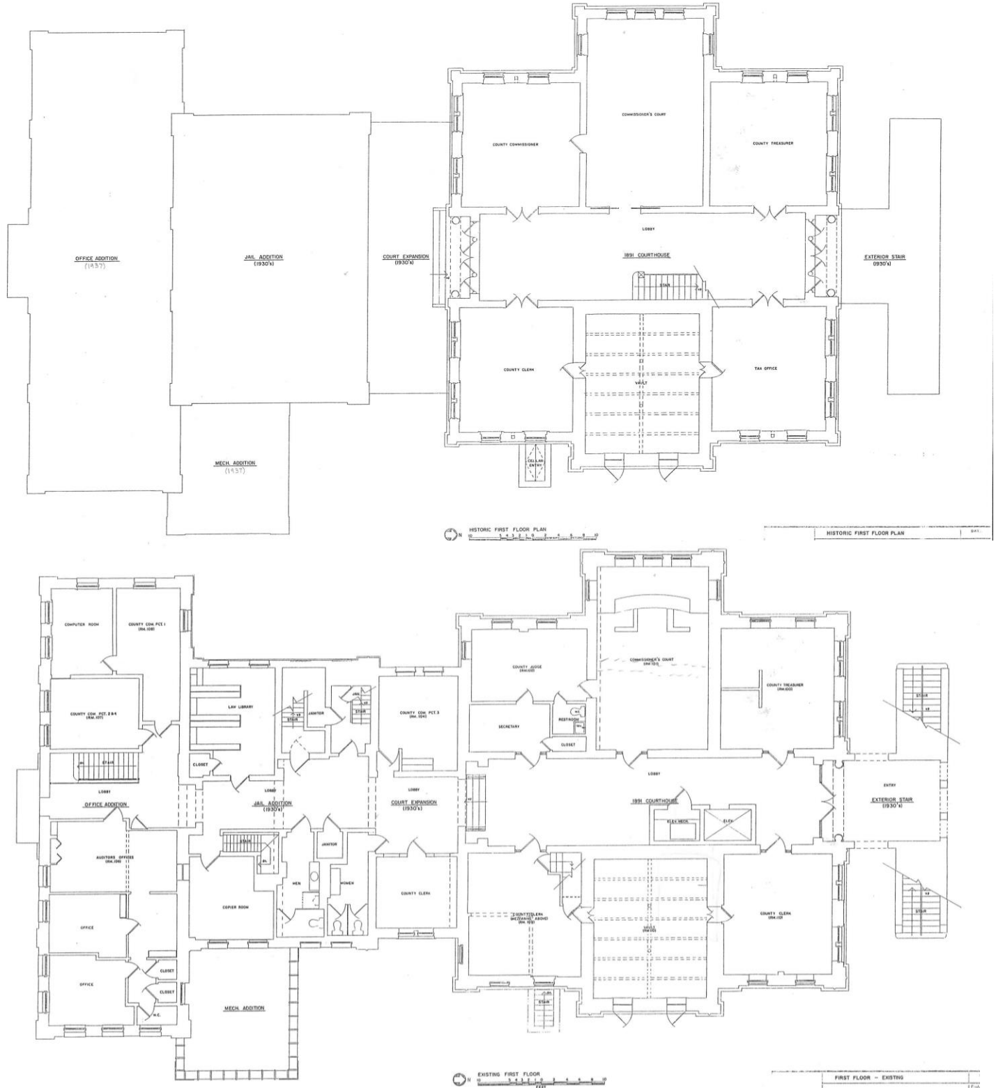
Figures 8 and 9: Historic (top) and existing (bottom) first floor plans. Drawings from Luhn's Master Plan for Restoration/Renovation of the 1891/1935 Tyler County Courthouse (2000).
