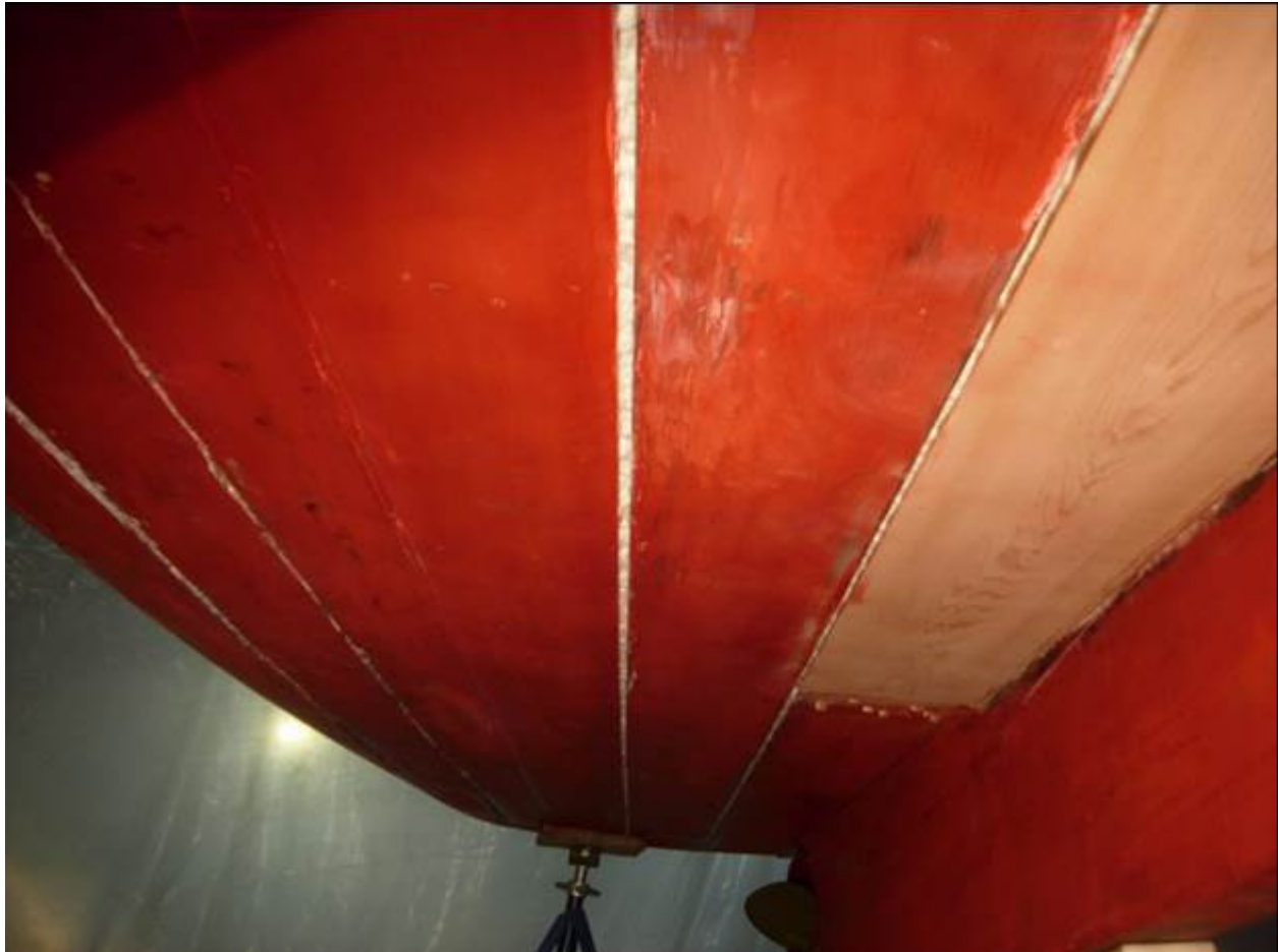
MT_GlacierCounty_Rising Wolf_0011, new garboard plank cotton seams.
