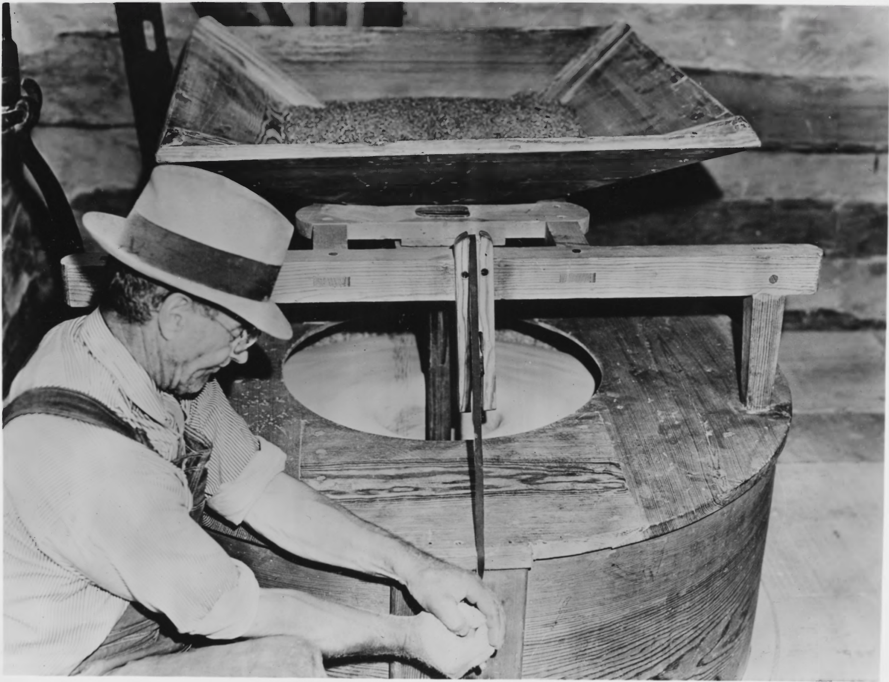
Wheat Burrstones in motion. Second Floor of Mill. Miller regulating flow of wheat from Hopper to Stones.
