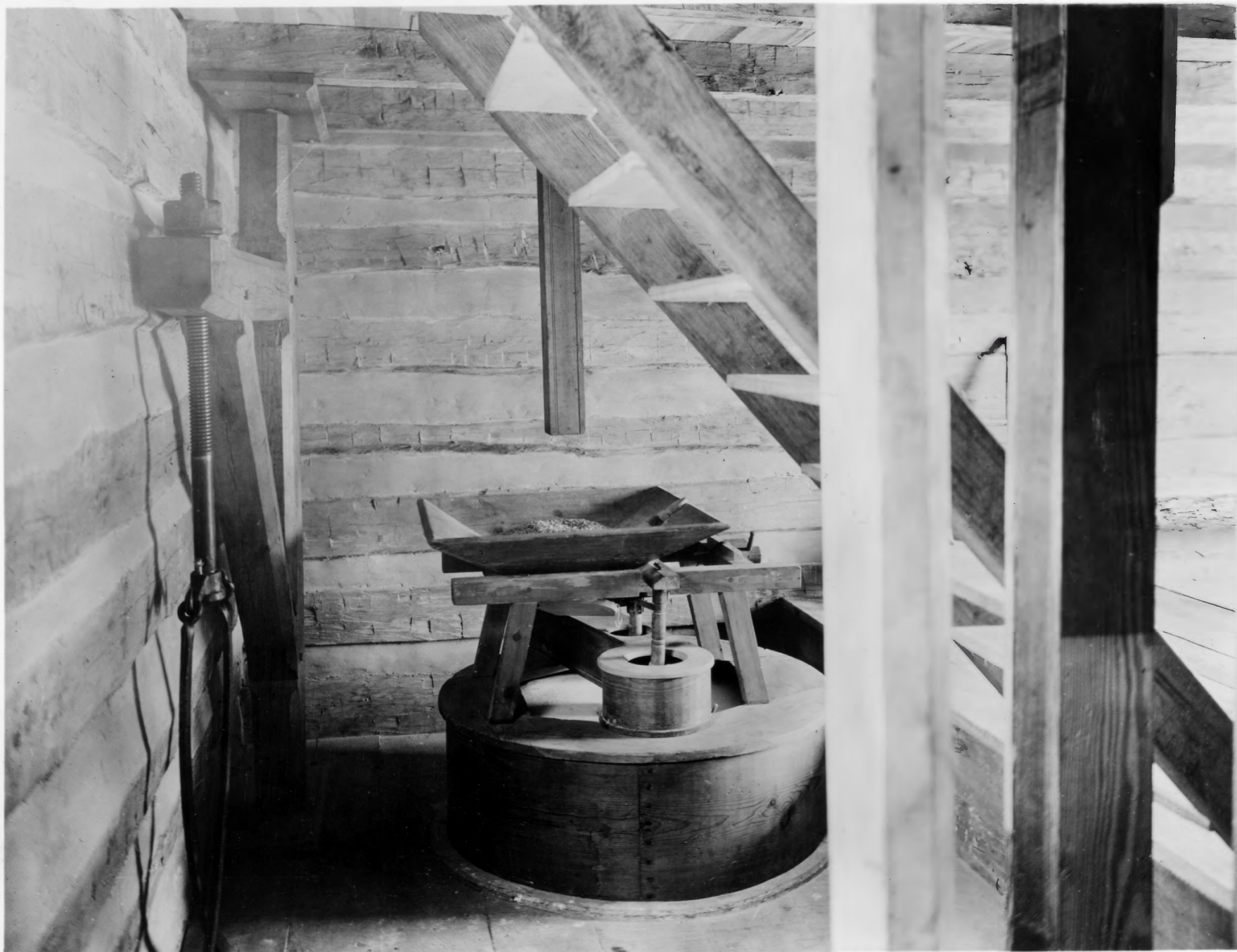
Corner of Mill, Second Floor, showing Corn Burrs and Apparatus. Note on left the Crane used to raise and lower the stones for sharpening. On the right, stairway to Third Floor. Right foreground note Elevator Chutes.
