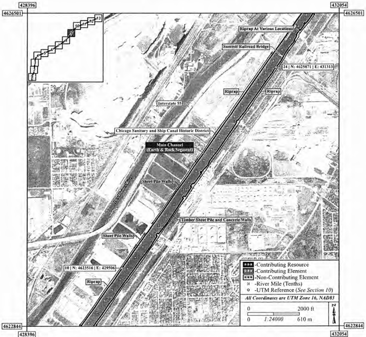
Figure 2.9: Scale map of a portion of the Chicago Sanitary and Ship Canal Historic District.
