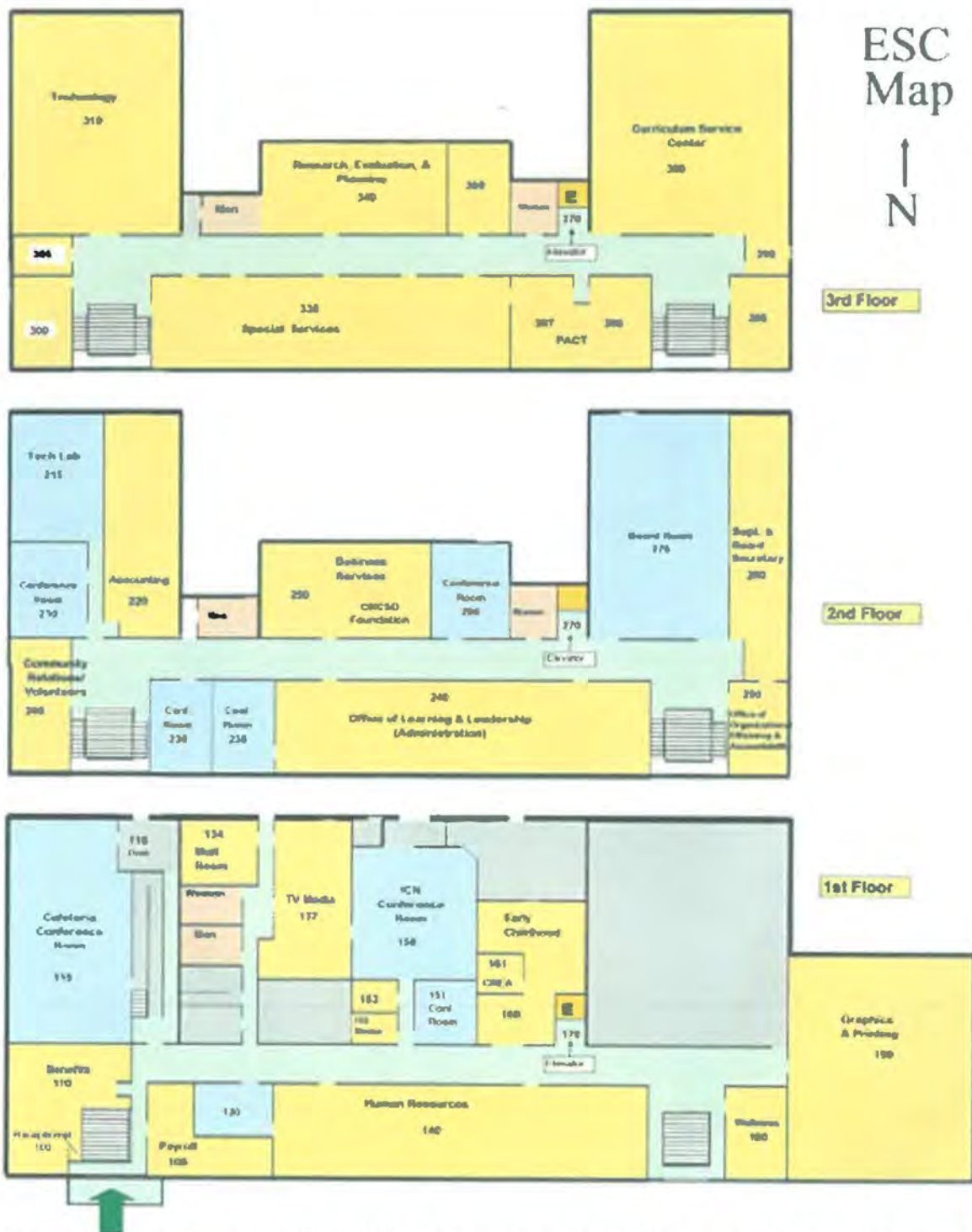
Floor plan of Grant just before the 2008 flood (color code is not known). Note that that the former class rooms located at the base of the "U" shape on either side of the central corridor have few partition walls. Where there are walls, most are not located in the same places as the original walls. Collection of Jo Ellen Johnson.
