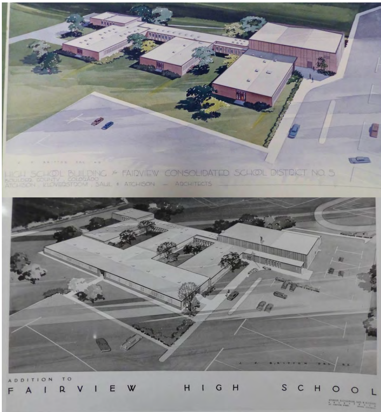
Figure 13. Fairview High School, Boulder County by Atchison Kloverstrom. Top drawing (1960) shows original design for school with finger plan. Second drawings (1962) shows addition closing off the finger plan. (Boulder Valley School District files).
