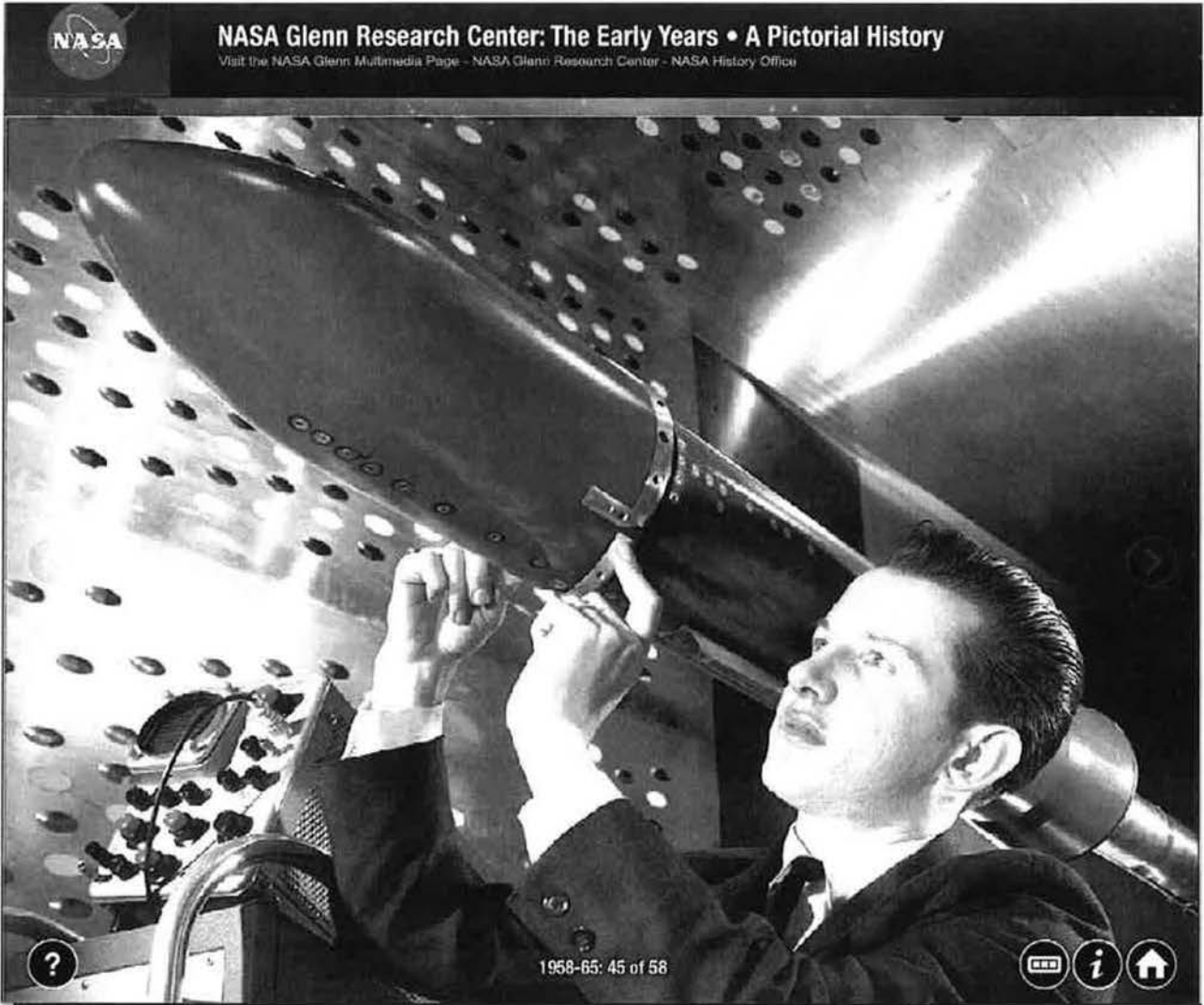
FIGURE 15 – Scale Model of the Agena/Mariner C spacecraft in the 8- by 6-Foot Supersonic Wind Tunnel at NASA Lewis Research Center, March 18, 1964; NASA, Photo C1964-68848, NASA Glenn Research Center: The Early Years - A Pictorial History, http://www.grc.nasa.gov/WWW/portal/gallery .
