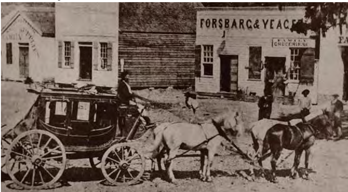
Figure 11. The so called “mud wagon,” preferred across much of the south where road conditions were often poor and difficult to navigate.
