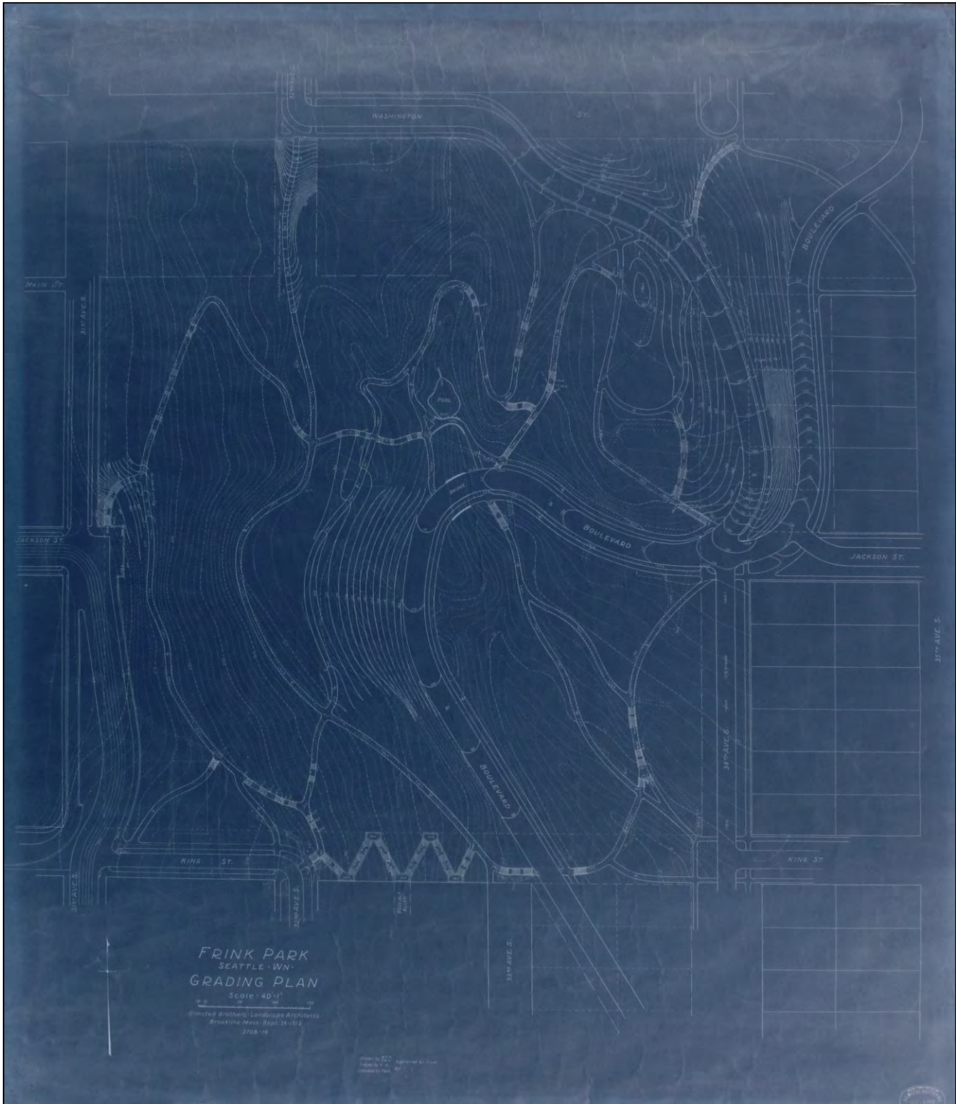
"Frink Park Grading Plan" showing proposed construction of pathways and steps, September 24, 1912, Olmsted Brothers (Seattle Municipal Archives [SMA], item no. 2330).
