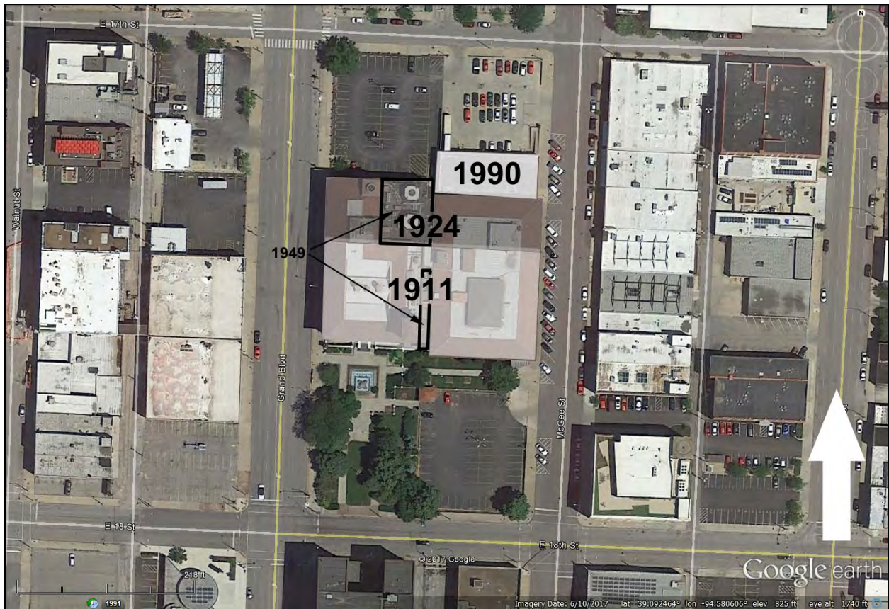
Figure 31. Site plan annotated with dates of construction. The 1949 addition filled in the U at the north end of the building at levels one to two and added a second and third story at the area between the east and west wings. Source: Google Maps, 2017.
