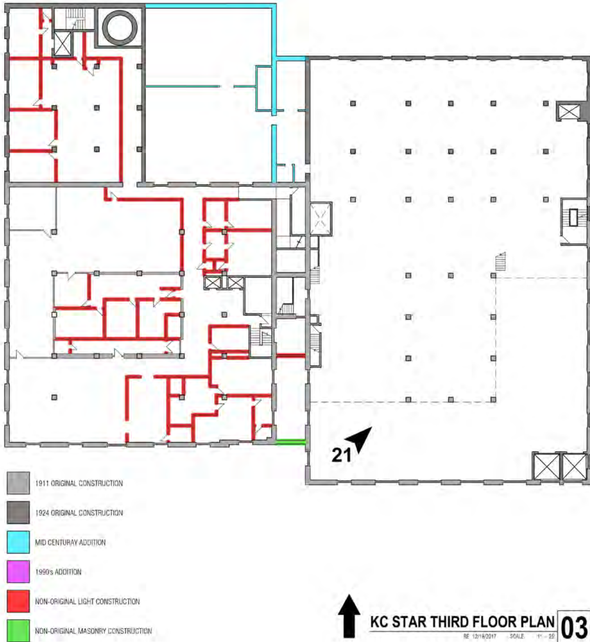
Figure 8. Photo map: Third Floor. Source: Generator Studio, "Kansas City Star As-Builts," 2017.
