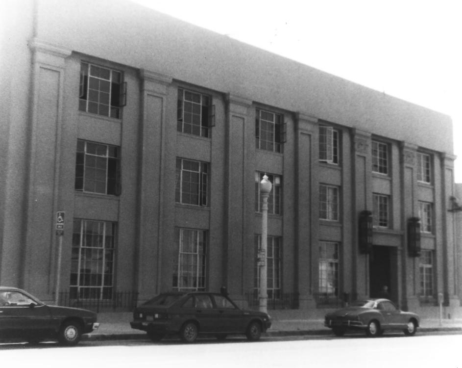
Eagles Hall, 733 8th Avenue, San Diego. Photograph taken June 15, 1984 by Ray Brandes, 2725 Barnson Place, San Diego, CA 92103. Photograph taken from west looking to east. The expanded facade of 1934 is of concrete block covered with sand-textured stucco. Photograph 5 of 10 photographs.
