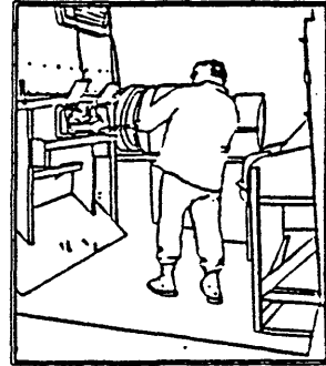
CUT NAILS ARE SHOVELED BY HAND INTO RETORT TUBES.
