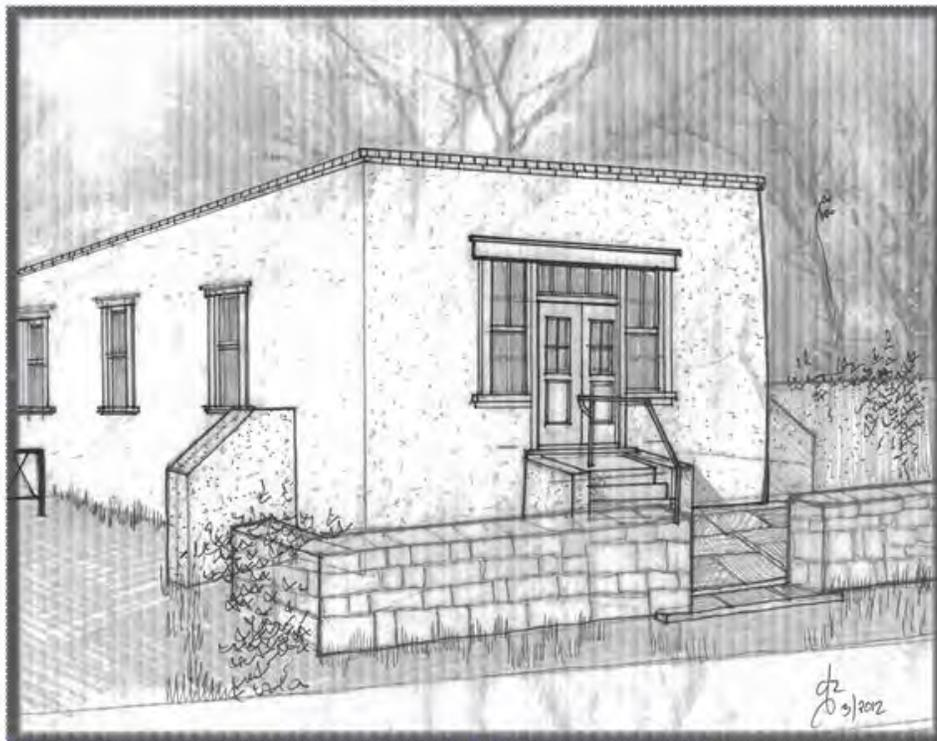
Figure 2: Existing east and partial south elevations based on 2012 overlay photo perspective. Note the front masonry wall and concrete buttresses have been removed as part of the 2013-2014 restoration. Courtesy Dale F. Zinn and Associates.
