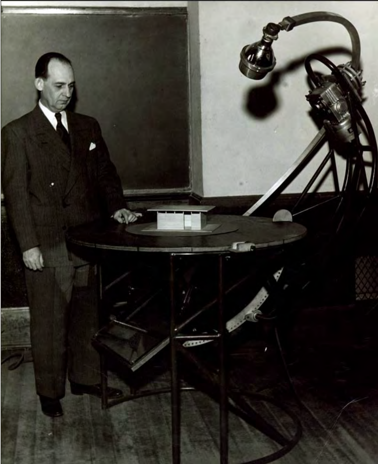
Figure 7. George Beal demonstrating his Inside-Outside Heliodon, 1953. Photo from: http://lawrencemodern.com/bakers-dozen/university-place/heliodon/ .
