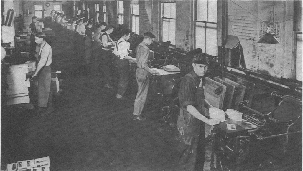
Murphy Co. job presses used to print smaller illustrations are lined up in this 1912 photograph. (Purcell, 173)
