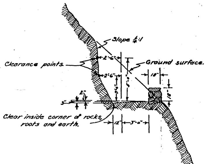
TRAIL SECTION IN SOLID ROCK WITH PARAPET
