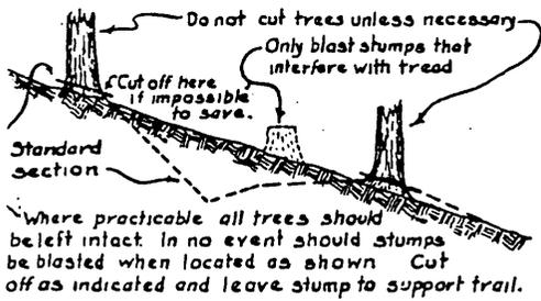
FIG. 1. BLASTING STUMPS
