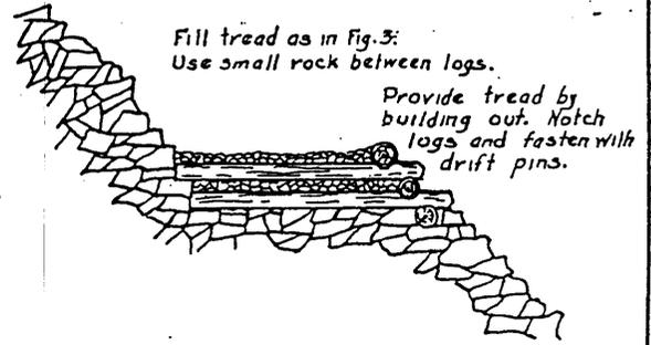
FIG. 4. LOG CRIB ON RUBBLE
