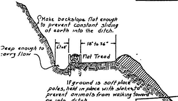
FIG. 6. TRAIL WITH DRAINAGE DITCH
