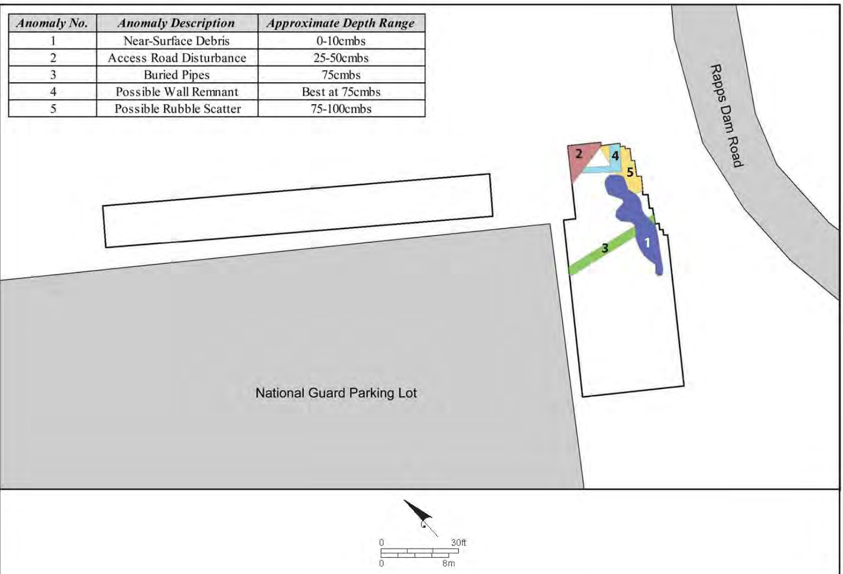
Figure 13: Geophysical anomalies detected during GPR survey of Area 2 and Area 3.
