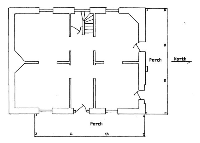
Scale 1/8" = 1 foot, slightly enlarged by Xeroxing. Outside dimensions of the structure excluding porches are 28'x36'.
