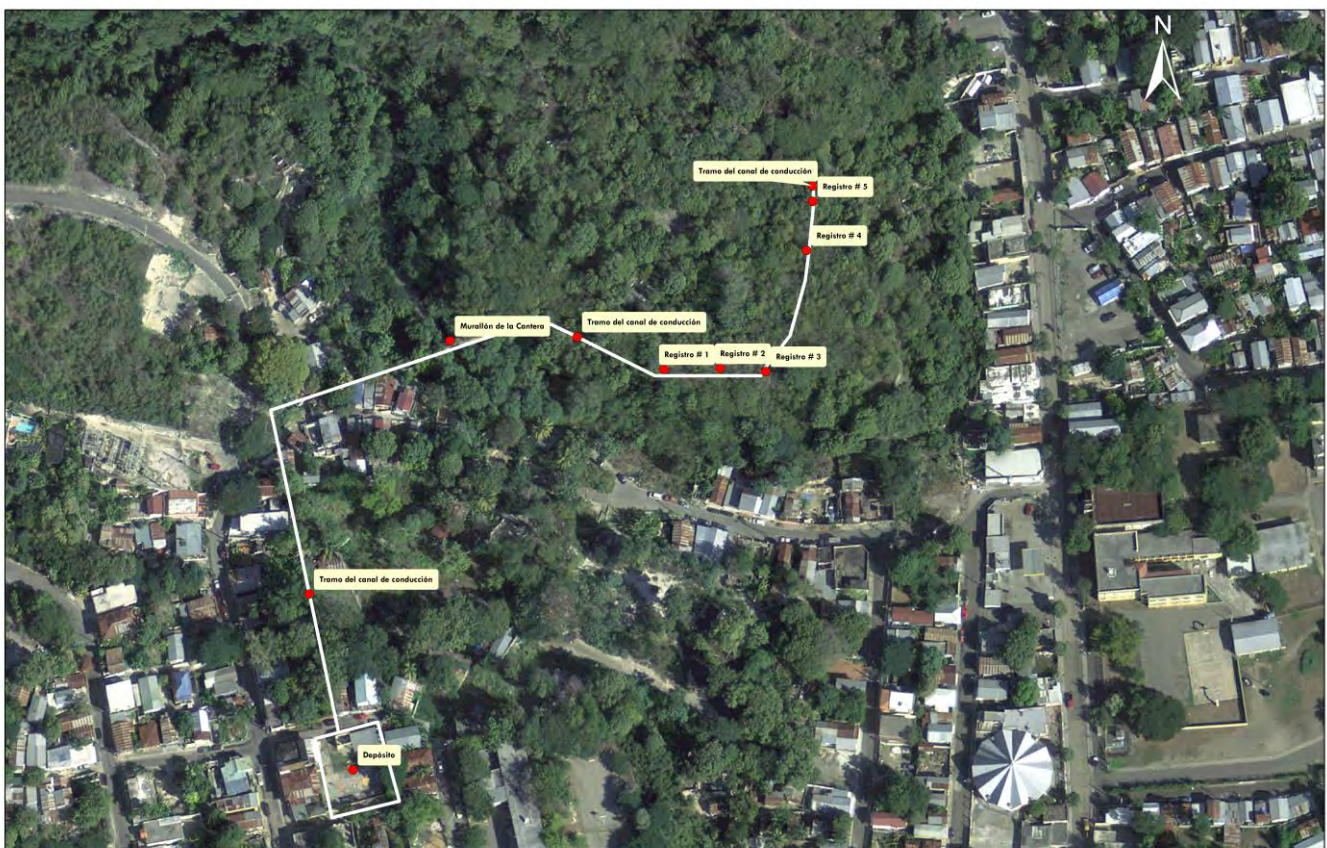
Figure 1. Alfonso XII’s extant components. The conduit channel runs through private backyards today. At some points, the top portion of its vaulted shape surfaces above ground, allowing to determine its traverse course from the western end of the Murallón de la Cantera to the deposit’s entrance. The points within the tree line (conduit channel and manholes) were found by PRSHPO personnel. (Map prepared by Eduardo Cancio, PRSHPO, 2019).
