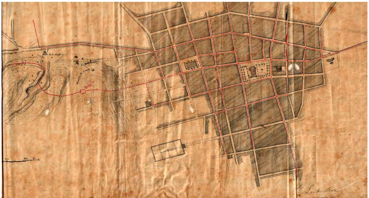
Figure 18. The image above depicts in red the aqueduct's cast iron pipe network from the deposit throughout the city.
