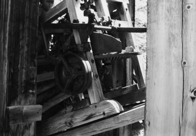
Figure 11: Feature 8, the gear mechanism which fed the ore from the hopper into the trough below the stamps. The picture was made from the east side of the mill looking into the machinery.
