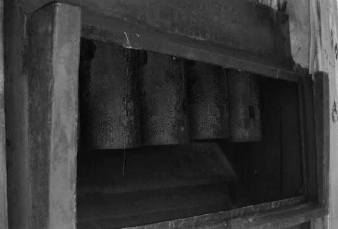
Figure 10: Feature 8, the stamps. This photograph was taken from the west side of the mill looking directly into the machinery. Only four of the five stamps are visible in this view. The trough is directly below the stamps.
