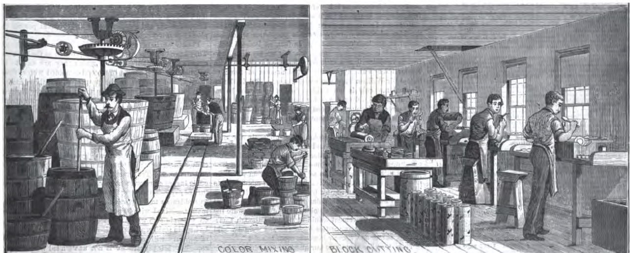
Figure 22 – Here Scientific American illustrates the color mixing and block cutting rooms in a wallpaper factory. These stages of the wallpaper manufacturing process would have looked much the same in the Howell & Brothers' Washington Avenue factory (from the July 24, 1880 issue of Scientific American ).
