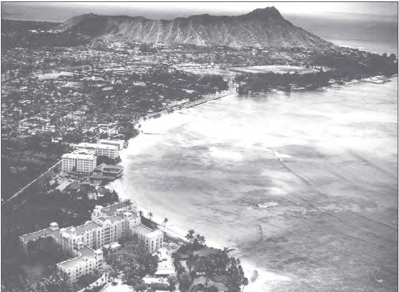
Source: DLNR Waikiki Beach, Oahu, Hawaii: History of its transformation from a natural to an urban shore. Page 13: Caption on photo “Figure 11. Aerial photo, circa 1940, looking toward Diamond Head; Royal Hawaiian-Moana Hotels Beach (curved groin near bottom); Kuhio Beach; “crib wall’ breakwater; seawall along section of Kalakaua Ave.; Natatorium in distance at top right. (By Anon)
