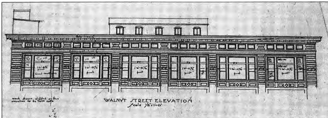
Figure 2: Added sixth floor, south elevation, east building (original plans, architects Proudfoot and Bird, Sheet 10, undated)
