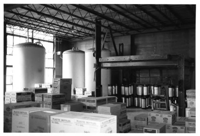
Grand Canvon Power House interior. Tanks and heavy steel work on the right are original. Space framing and wood decking above are recent additions, but are totally removable and are not attached to the structure.
