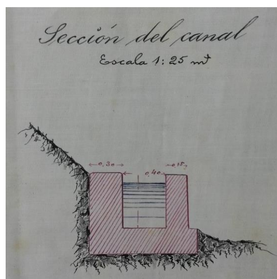
Figure 6. Above, Desideria's general plan, showing the dam, canal (in red), coffee factory and drainage trench. Below, details of the dam, a dam's transversal view and a section of the masonry canal with height and width.
