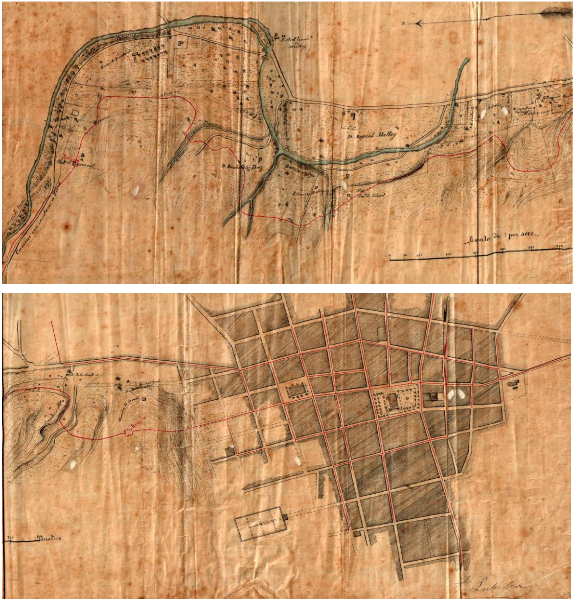
Figure 21. The upper image of the 1875 map prepared by Timoteo Lubelza shows the canal's route (in red) from the intake in the Portugués River, along Ponce's north outskirts, towards the deposit. The image below depicts the aqueduct's pipe network from the deposit throughout the city (also in red)
