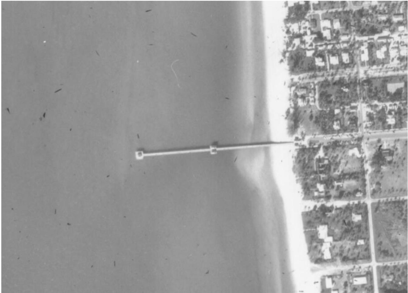
Figure 1: December 1962 Aerial view of the Naples Pier showing the post-Hurricane Donna design of the pier. Clearly visible are the paired rectangular pavilions at the shore and midpoint of the pier, and the single pavilion at the end of the pier.
