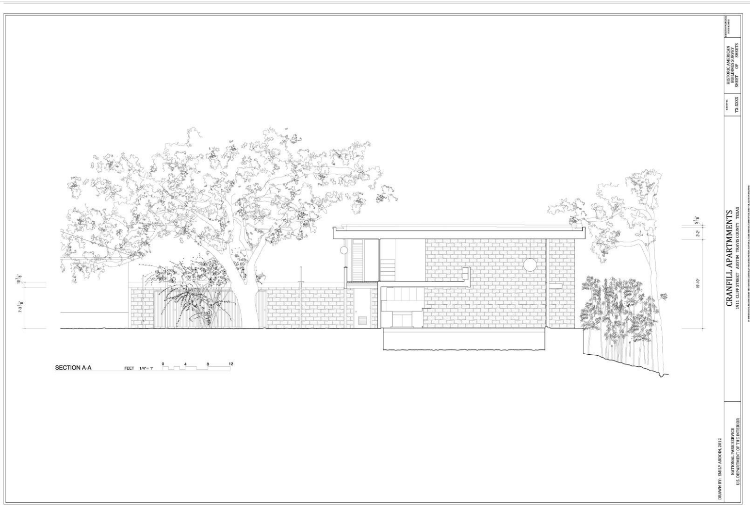
Figure 4: Building section through Unit 3 drawn by Emily Ardoin for HABS from field measurements.
