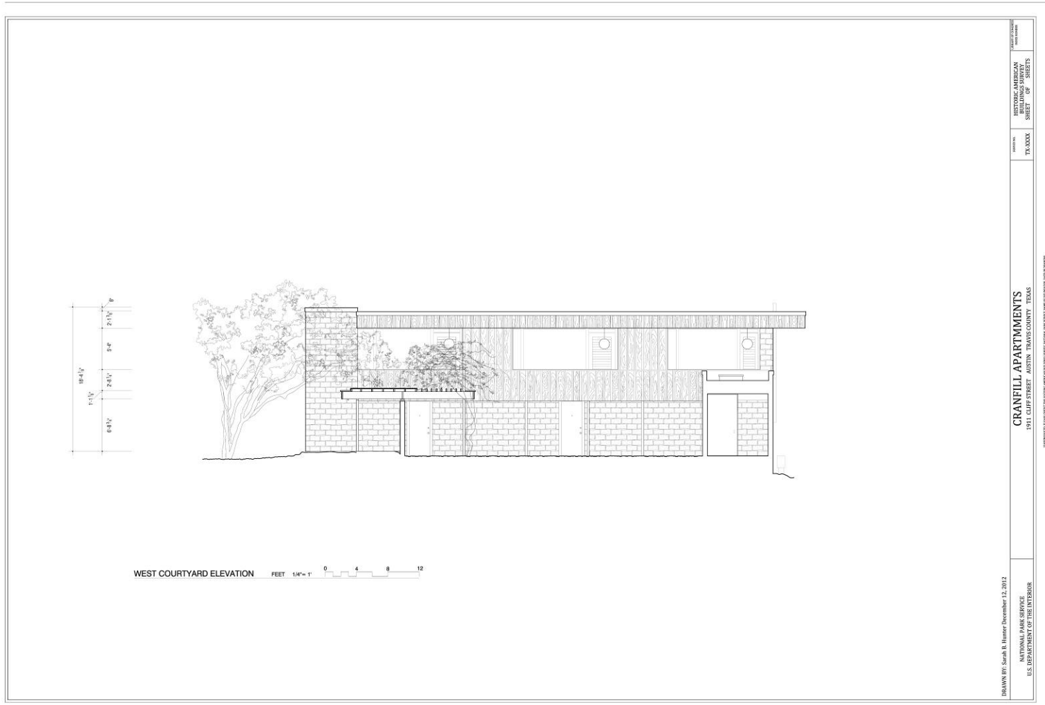
Figure 5: West exterior elevation drawn by Sarah Hunter for HABS from field measurements.
