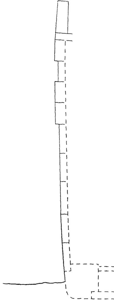
Figure 4: A section of the *O. J. Walker's* hull (drawn by Joseph R. Cozzi, 1995).
