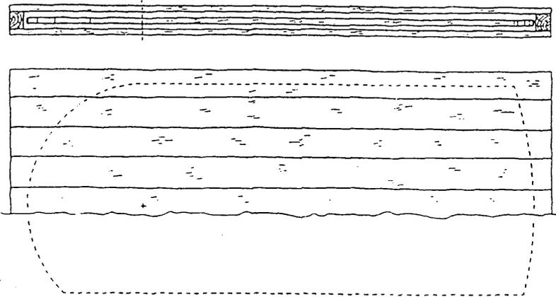
Figure 5: The *O. J. Walker's* centerboard trunk with the centerboard outlined in a dashed line (drawn by Joseph R. Cozzi, 1995).
