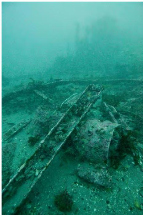
Figure 003. Depth charge rails and depth charges can be found at the HMT BEDFORDSHIRE's stern (Joe Hoyt, *Monitor* National Marine Sanctuary).
