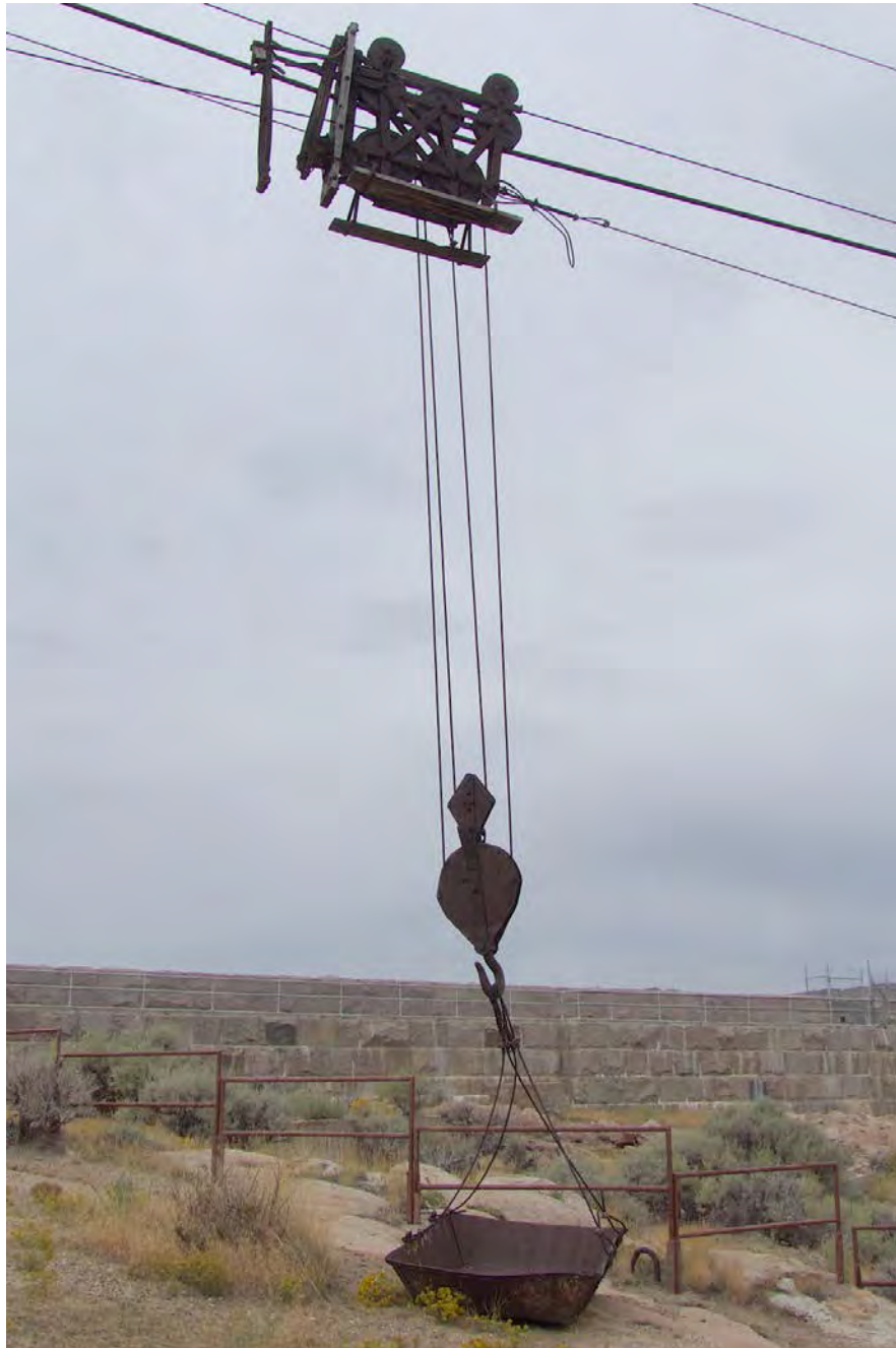
Photo #48: Detail of cableway bucket, hook, and carriage assembly (contributing). Camera facing west.
