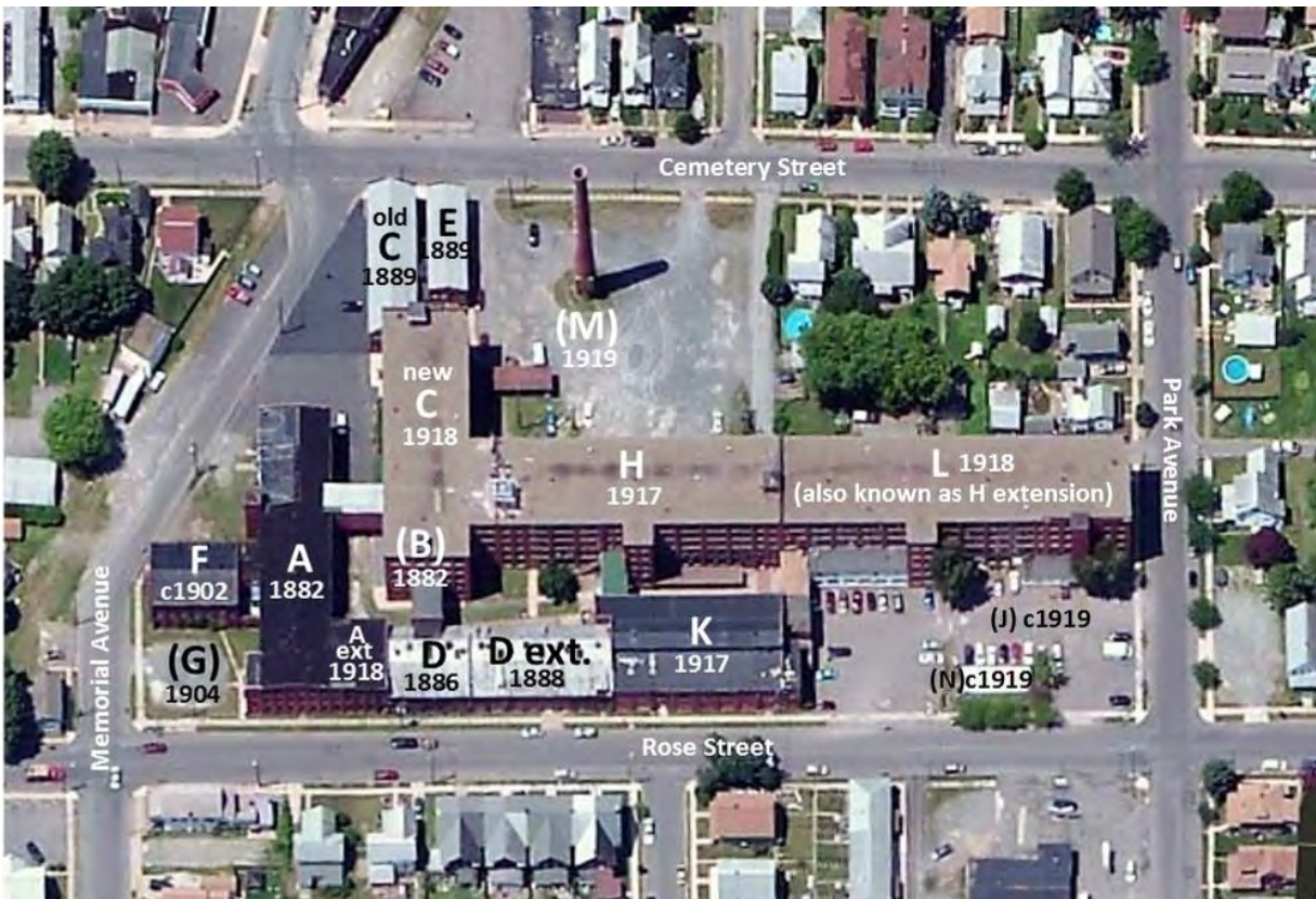
Figure 12. Site plan of the Lycoming Rubber Company factory showing buildings and the date they were constructed. Buildings noted in parentheses were demolished by previous owners. Buildings noted as “old C” & “E” are owned by Weldon Factory Sales Room, Inc., all others owned by PJ Holdings. Map created by author from Bing Maps.
