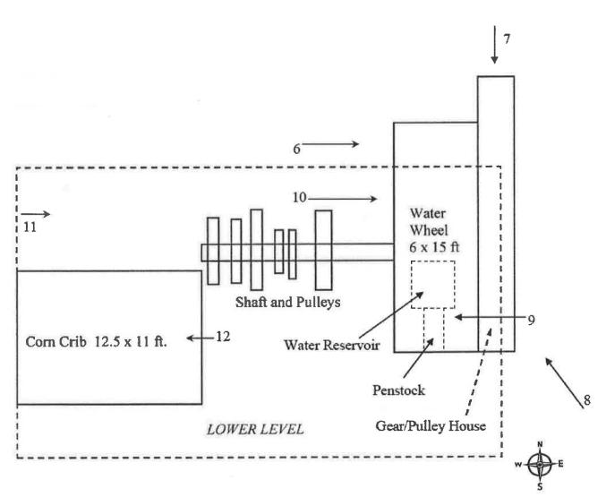
Lower Level of the Bodenham Mill (not to scale)
