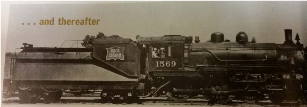
HP3 – An example of a semi-Vanderbilt tender that expanded the base of the cylindrical original tank with sloping sides down to the frame. From Ed Wojtas, "Rock Island's Very Own Tenders," Trains: The Magazine of Railroading , July 1969, p. 46.
