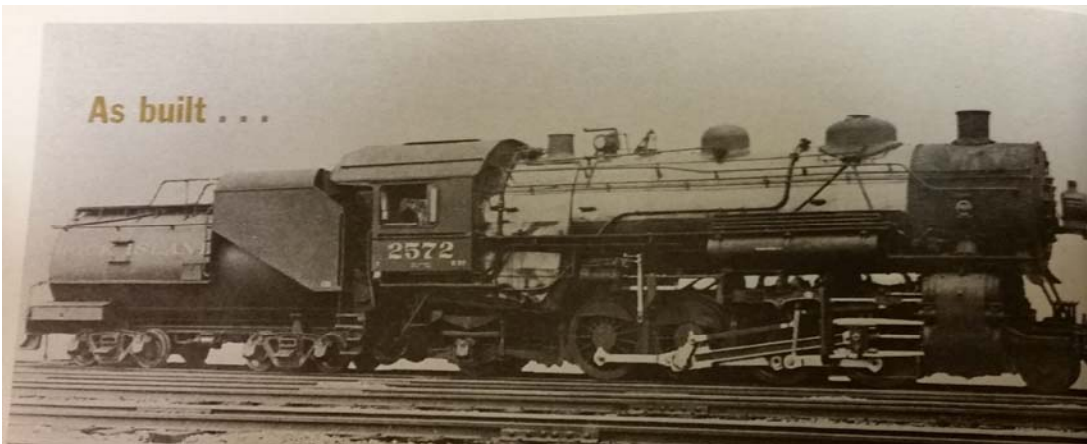
HP2 – An example of a Vanderbilt tender, with cylindrical tank on its side. From Ed Wojtas, "Rock Island's Very Own Tenders," Trains: The Magazine of Railroad ing. July 1969, p. 46.
