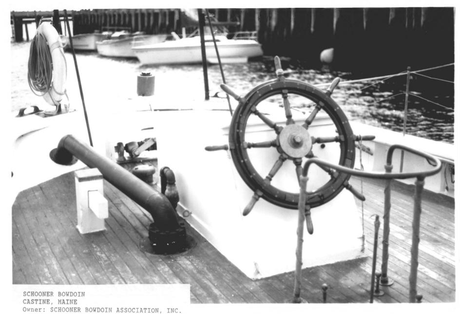
VIEW OF POOP, SHOWING THE WHEEL, BOX, & ENGINE EXHAUST.
