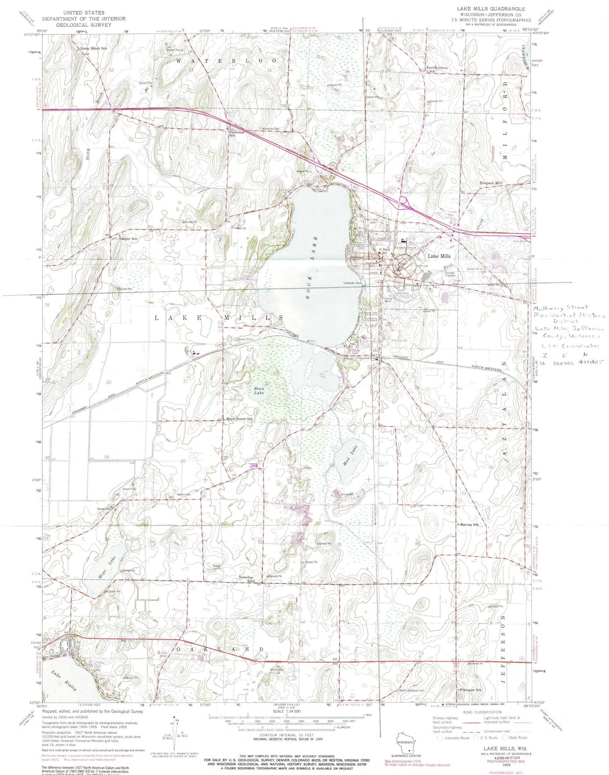
The difference between 1927 North American Datum and North American Datum of 1983 (NAD 83) for 7.5-minute intersections is given in USGS Bulletin 1875. The NAD 83 is shown by dashed corner ticks
