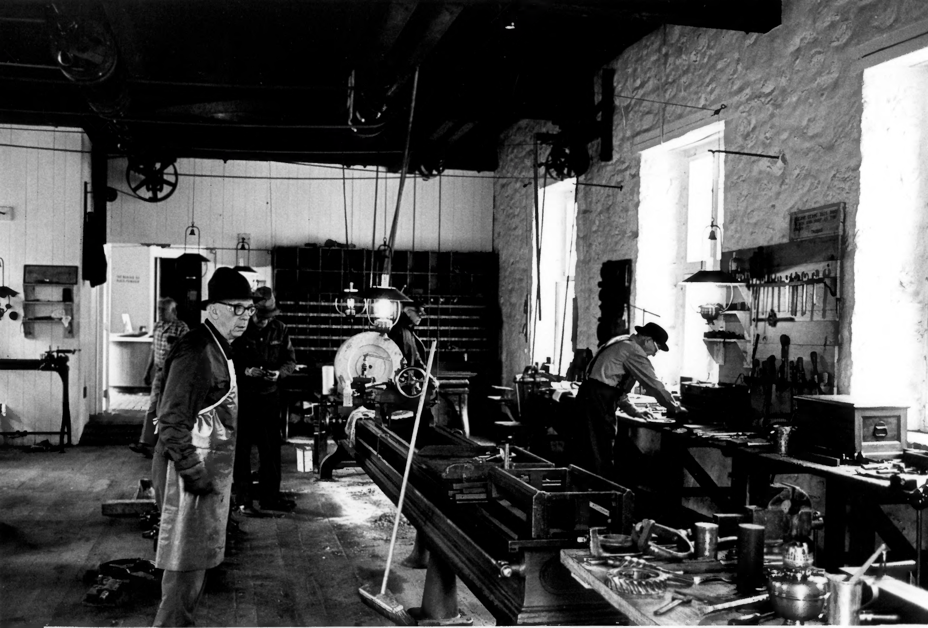
S-8. Interior. Restored machine shop with operating 19th century machinery powered by shafts and belts. Award-winning volunteers demonstrate daily for visitors.
